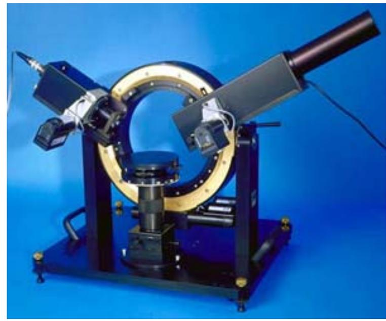
Fig 13. Ellipsometer Equipment
